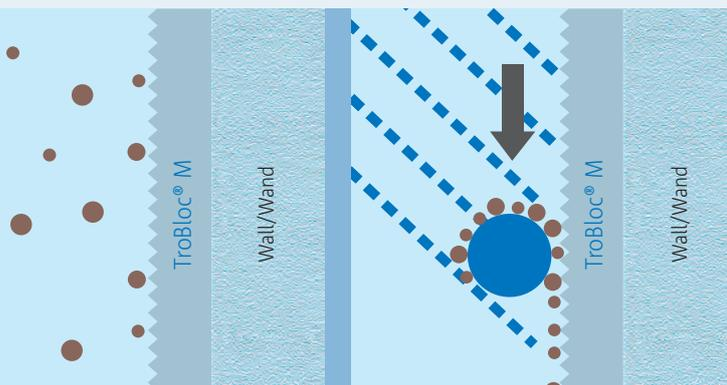
Easy-to-clean-effect: With TroBloc® M, even large surface areas can be cleaned fast; fluid runs off immediately, taking adherent substances and particles with it, due to the specially designed surface.
