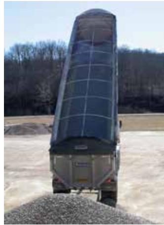
Professional lining: Z-sheets attached to the truck bed prevent material from drifting under the lining sheet.
