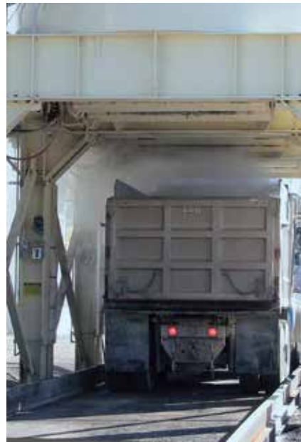
Emptying a bin: The Matrox lining of the bin ensures even and undisrupted loading of the bulk material.
