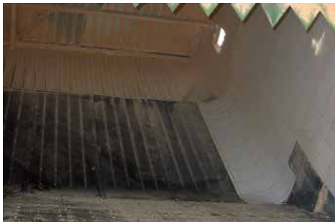
View into a hopper from below. With large-grained bulk goods, which may cause serious localised wear, lining the exposed parts with Matrox will considerably prolong the life span of the hopper.
