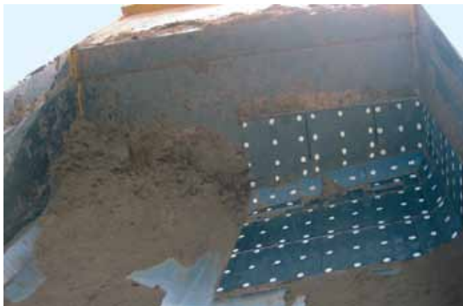
Comparison between Matrox and steel. The material adheres to large areas of the unlined steel surface. The area lined with Matrox is almost completely free.
