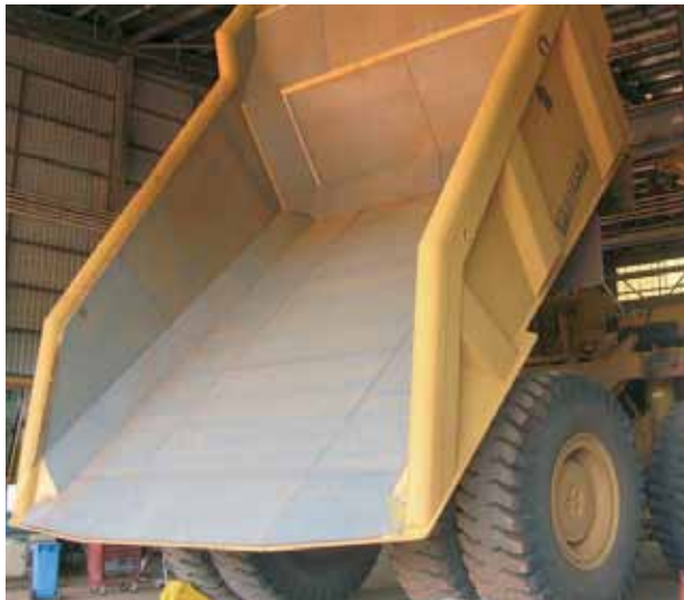
Matrox coils: Ideal for lining on road dump-truck beds.
